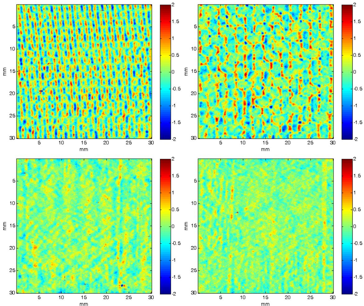
Fig 1. OptiTopo results: Upper left - 200 gsm glass roving fabric, upper right - 200 gsm carbon fiber roving woven cloth. Lower left - 100 gsm Spread Tow Fabric, lower right - 2 layers of 100 gsm Spread Tow Fabric. Color scale in  $\mu\text{m}$ .
