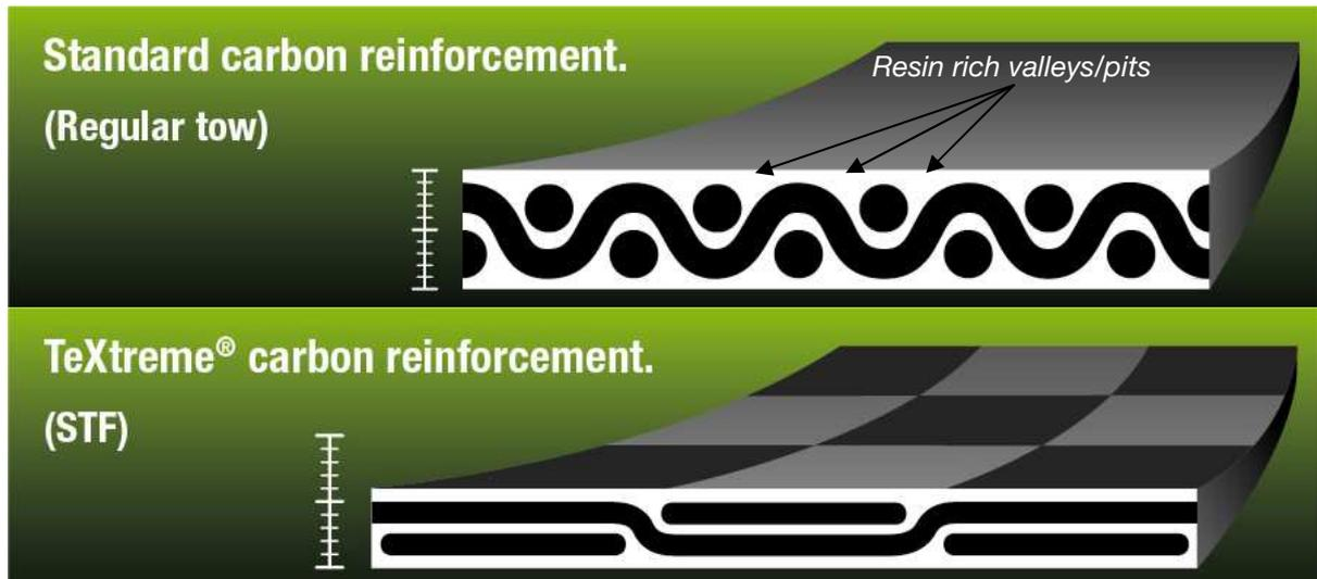
Fig 2. Spread Tow Fabrics (STF) reduces print through problem through its unique structure compared to standard carbon reinforcements.
