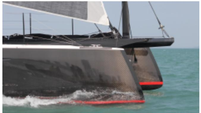
**Left/above:** fabric patterning that you can be proud of... the first of the HH66 Morrelli&Melvin-designed luxury performance cats built at Hudson Marine under the supervision of Paul Hakes shows off the quality of the finished appearance using precisely and finely woven TeXtreme carbon fabrics. The TeXtreme solution is already in common use in racecars, aerospace and military applications
